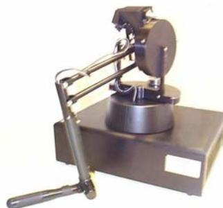
Figura 5.6: *PHANToM* Premium 1.0 (a) y *PHANToM* 1.5/6DOF (b).
