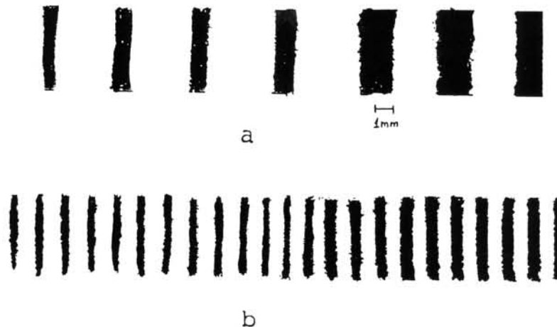
Fig. 2. Pattern for (a) gravity waves (15 Hz, dominance = 0.4) (b) capillary waves (50 Hz, dominance = 5). Dominance is the square of the wave number relative to the capillary wave number.
