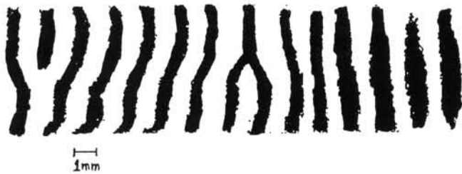
Fig. 6. A couple of defects at a driving frequency of 50 Hz.
