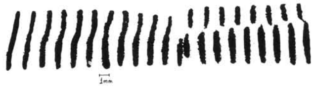
Fig. 7. Formation of a defects' line (right) from an undulated structure (left).
