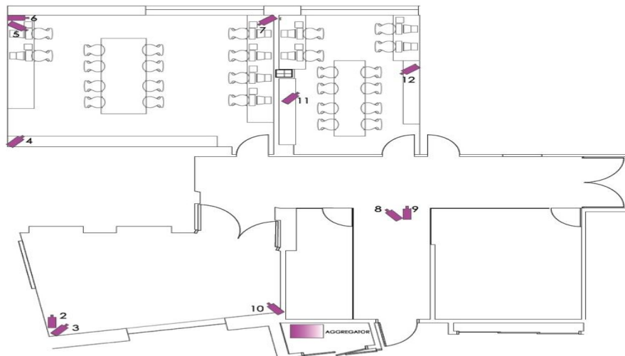
Fig. 11: Installed Occupancy Sensors (CUN, Phase 1)
