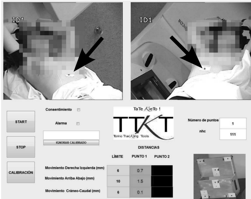
FIG. 4. A view of the user interface of the program. The algorithm is tracking the motion of only one point placed on the patient skin (black arrow). Motion magnitudes in mm are shown besides their respective tolerances; they are depicted over green color if tolerances are being met, or over yellow or red colors otherwise.
