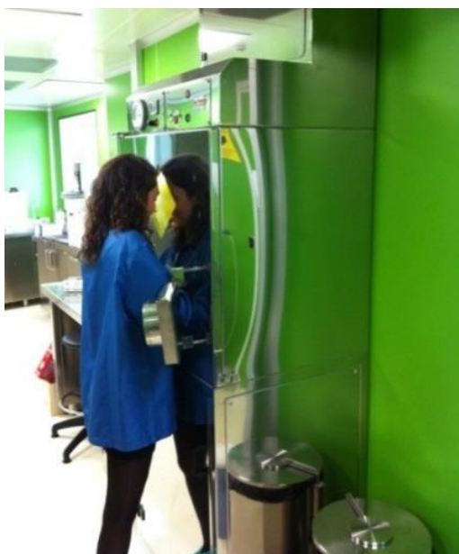
Figure 13: Hot cell installed in the Molecular Imaging Unit of CIC biomaGUNE.
