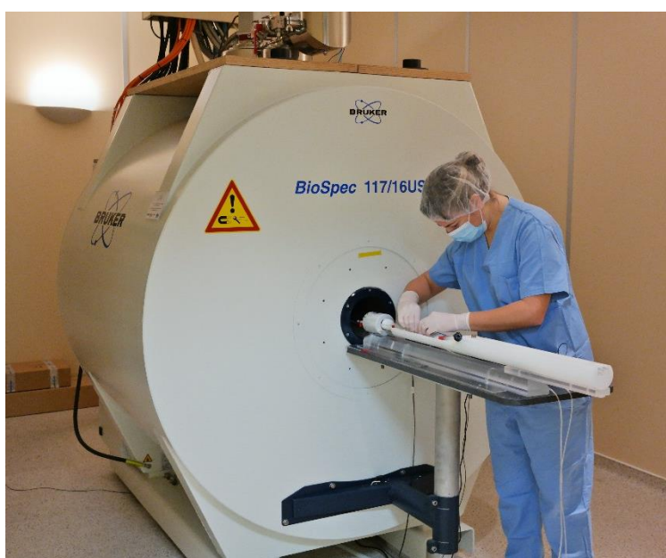
Figure 16: MRI 11.7 Tesla scanner from Bruker installed in CIC biomaGUNE.
