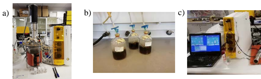
Figure 6. 2. 3-L fermentation reactor (a). Inoculation of Lactobacillus delbrueckii (b), monitoring and control system (c).
