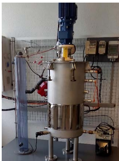
Figure 3. 2. Picture of the 80 L CSTR pilot-scale reactor that was used in batch mode for up-scaling.
