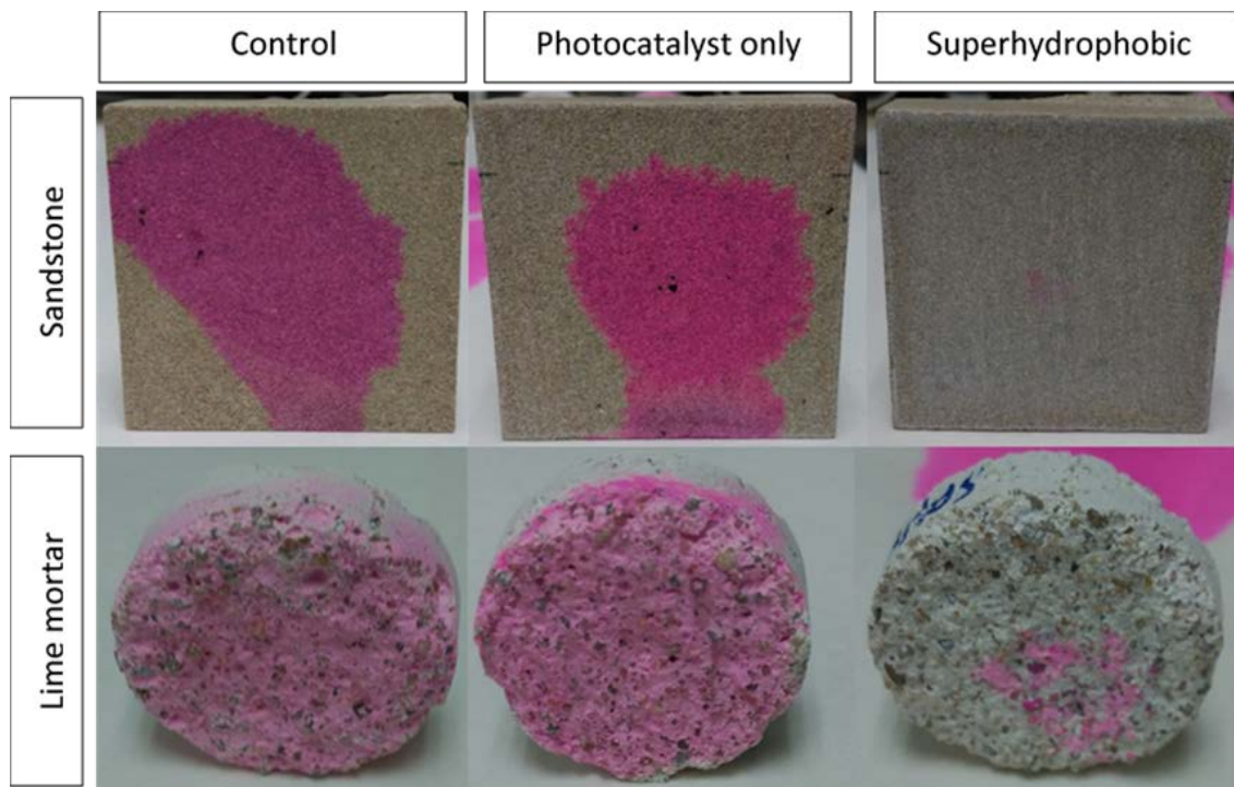
Figure 10. Results of the self-cleaning test for samples in vertical position: dye was deposited onto lime mortar and siliceous stone samples for one minute in horizontal position and then moved to vertical position.
