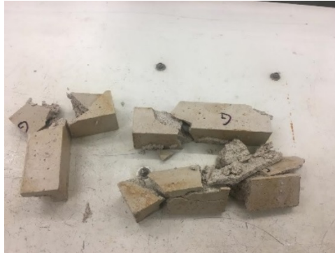
Figure 9. Pure air lime grouts subjected to one freezing-thawing cycle
