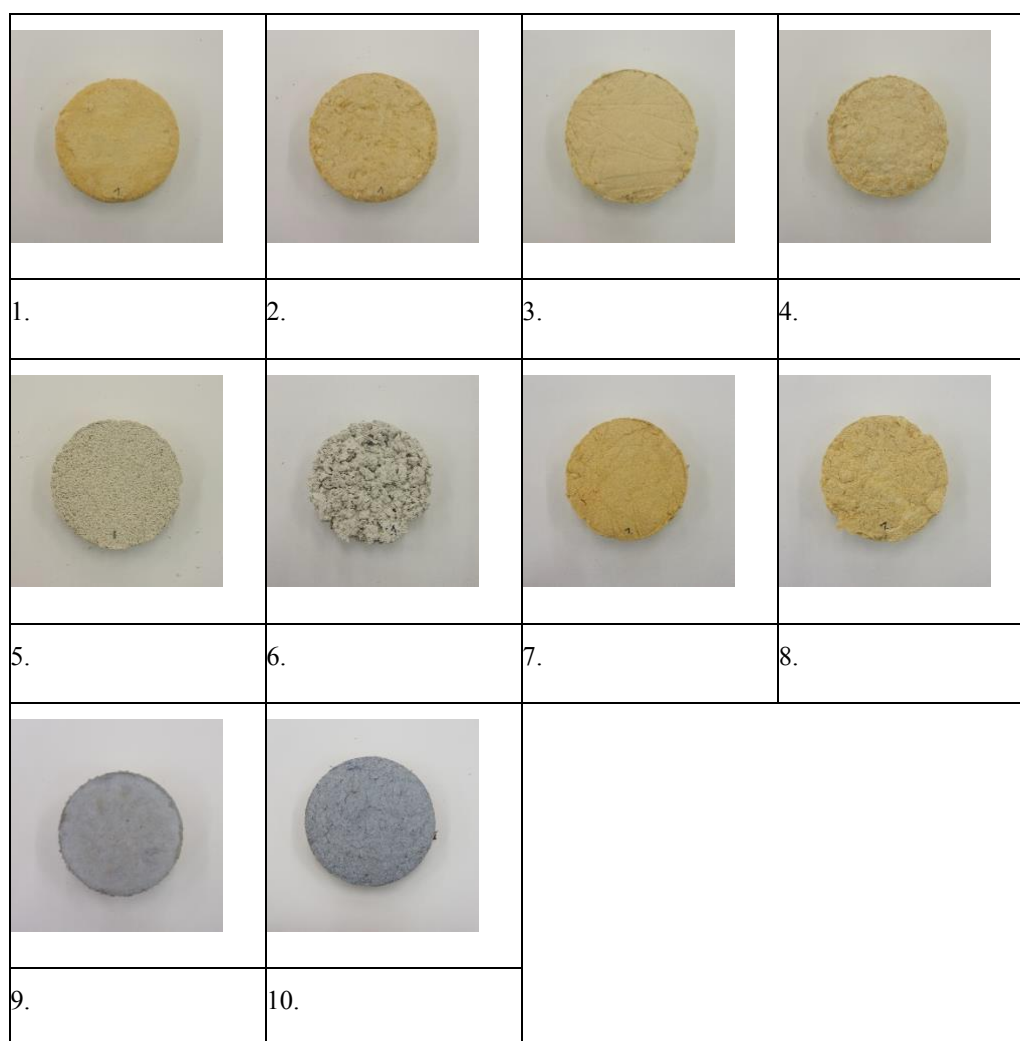
Figure 2. Samples for the tests of acoustic performance according to the standard UNE EN ISO 10534-2.
