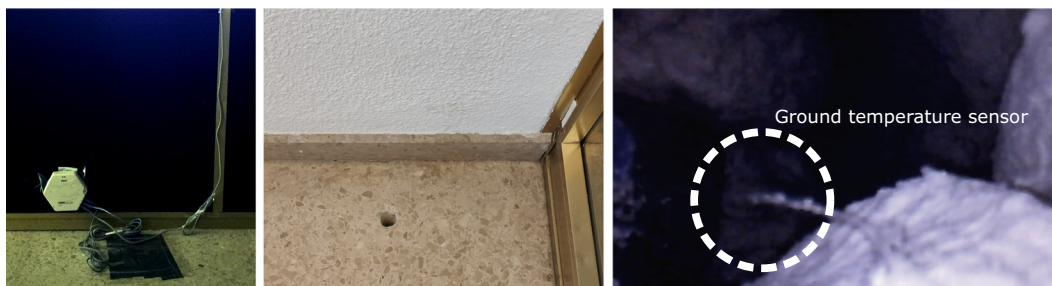
Fig. 8. sensors used to measure the interior and exterior surface temperatures of the slab in contact with the ground.
