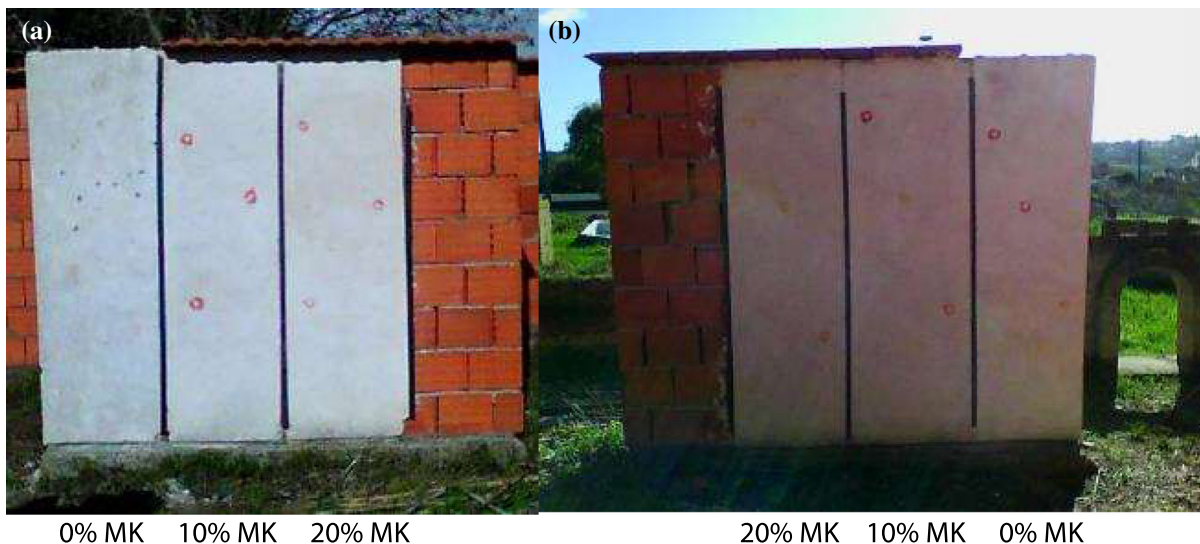
Fig. 4 Experimental pure air lime renders and air lime-metakaolin (MK) renders (marked with the percentage of MK replacing lime) after 7 years of natural exposure a South and b North, in a semi-urban environment 3 km from the Atlantic Ocean
