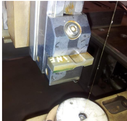
Figure 2. Slicing of one of the prisms to obtain tensile mini-samples.
